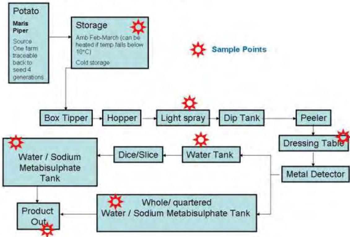
Schematic diagram of Solway Veg vegetable processing line and the points throughout this that were samples for potato metabolite analysis.
